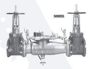
Series 5000SS Reduced Pressure Detector Assemblies are designed for use in accordance with water authority-containment programs. This series can be used to prevent the reverse flow of health hazard fire protection substances, i.e., glycerin wetting agents, foam agents, stagnant water, auxiliary supplies and water of non-potable quality from being pumped or siphoned into the potable water supply.
