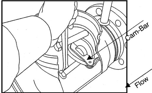
**3. Lift** the Check straight up and out of the port access hold.
