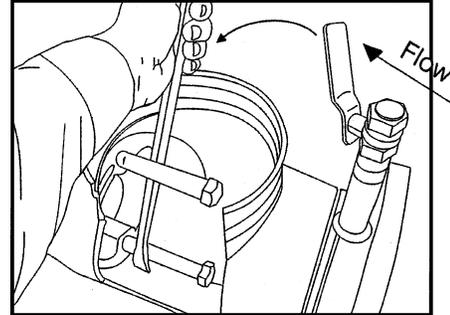
**5. Lift** the Check straight up and out of the port access hole.
