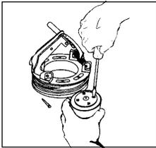
Before reinstallation of check assembly, thoroughly clean O-ring groove and lubricate O-ring with F.D.A. approved lubricant.
